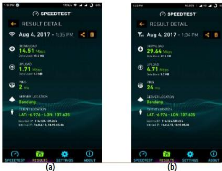
Fig 4. Data Download and Upload Speed Measurement Results for (a) Telkom's Indehome FTTH Network, (b) Telkomsel's 4G Network
