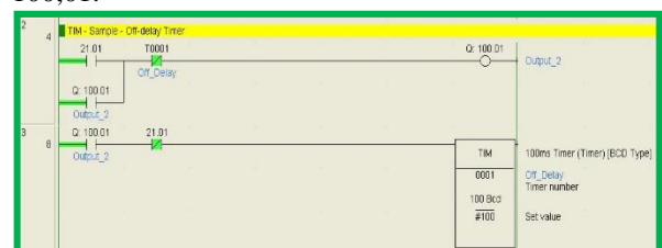
Gambar 7. Ladder program timer non-tunda
