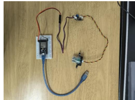
Gambar 17 Rangkaian Ujicoba Sensor Turbidity
