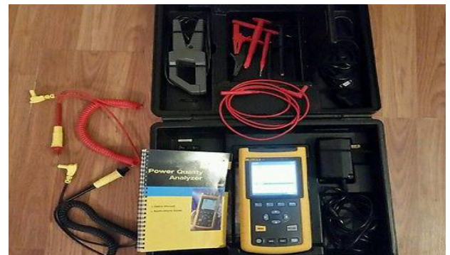
Gambar 3. Fluke Power Quality Analyzer 43B
