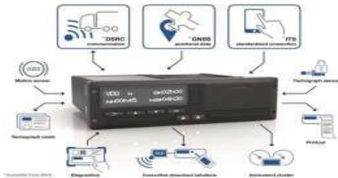
Gambar 1. Contoh Fungsi Fitur Smart Tachograph.
