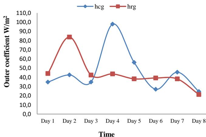
Gambar 4. Heat transfer coefficient data outside the evaporator
