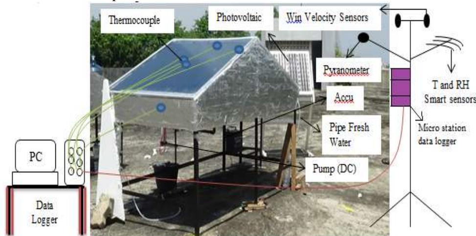
Gambar 1. Experimental Set up Desalination Tool
