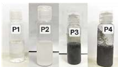
Gambar 4. Spesimen pelumas yang digunakan; P1: Polyolester (POE) oil, P2: POE + bacterial cel-lulose , P3: POE + carbon nanoparticles (graphene) , P4: POE + bacterial cellulose + carbon nano-particles (graphene)
