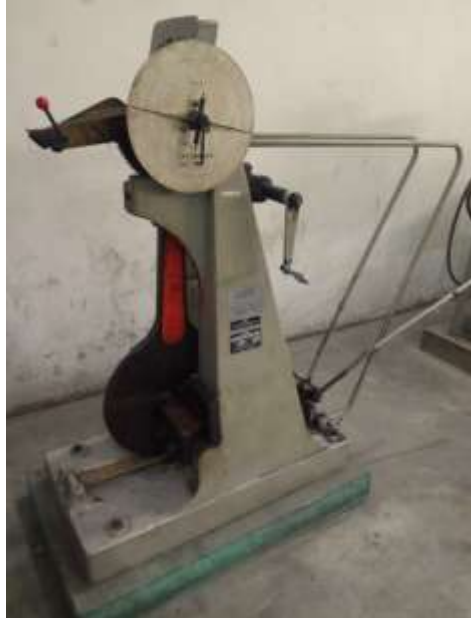
Gambar 5. Alat uji Charpy Impact Testing Machine type CI-30.
