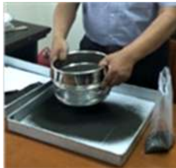
Figure 6. Iron Sand Sample Screening Process
