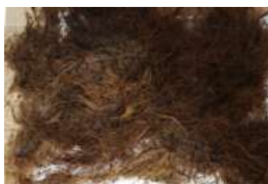
Figure 2. TKKS cellulose fiber after the delignification process (Thoriq et al. 2022)
