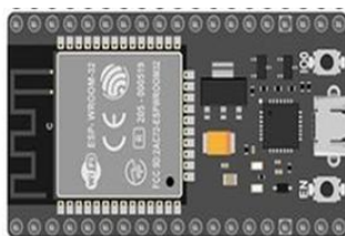
Fig. 1. ESP32 DevKit V1 Module - Microcontroller with Integrated WiFi and Bluetooth
