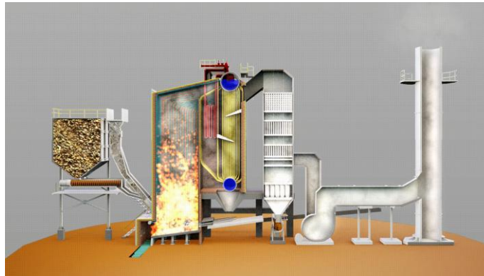
Gambar 3. Water Tube Boiler[7;15]
