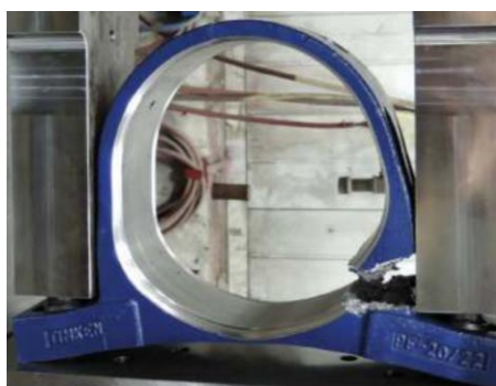
Figure 1. Failure modes of pillow block bearing housings [3].
