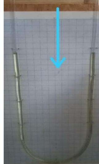
Gambar 6. Manometer pipa U
