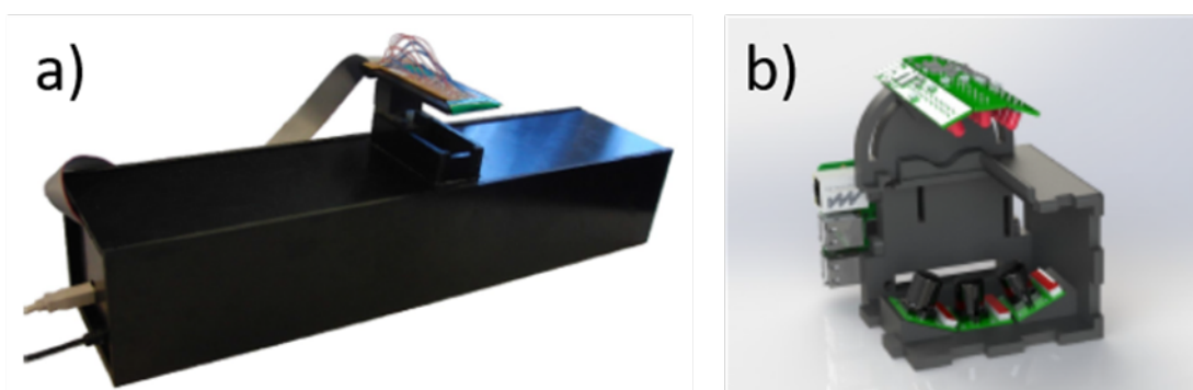
Fig. 4. Finger vein scanner of DMB group of the University of Twente using: a) high-end camera (UTFVPv1 [Ton and Veldhuis, 2013]) and b) low-cost camera (UTFVPv2 [Veldhuis et al., 2020]).
