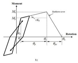
Figure 2. The structural model of school building: a) 3-D model of moment resisting frame with bracing to represent wall, and b) the backbone curve to represent the nonlinear material behavior of RC elements
